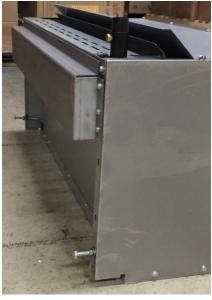
6. Wall mounting plate must be securely mounted and level at desired height, using (6) bolts or fasteners to be supplied by installer. Drill holes in mounting plate to match beam locations. Bolts must be secured to beam and wall and bolts must be rated to hold total load of 300 lbs. See below:
