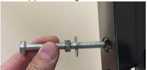
5. Completed Rear Bracket and leveling bolt installation below. Ready for mounting on wall plate.
